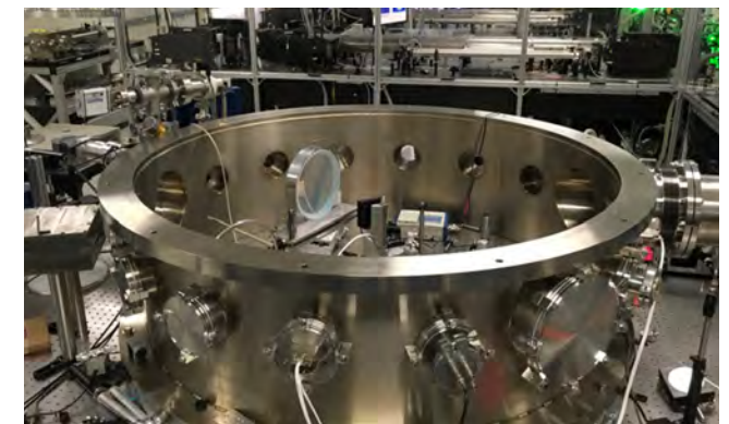
The target chamber (front) and ultra-high density laser (back) used in the micro-scale fusion experiments at CSU. Photo: CSU Advanced Beam Laboratory
